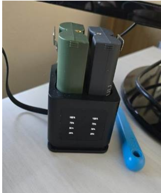
Battery charging dock and blue removal tool on Holly's desk. The front panel shows each battery's charge level: 100%, 75%, 50%, or 25%.
